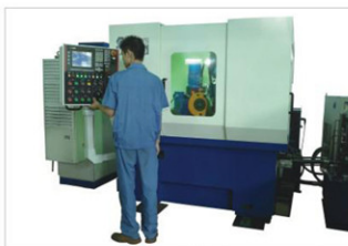
数控磨齿机 Numerical control gear grinding machine
